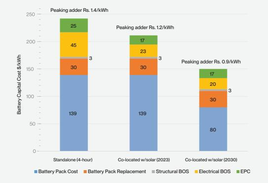
Storage cost can be lowered by co-locating batteries with solar plant
