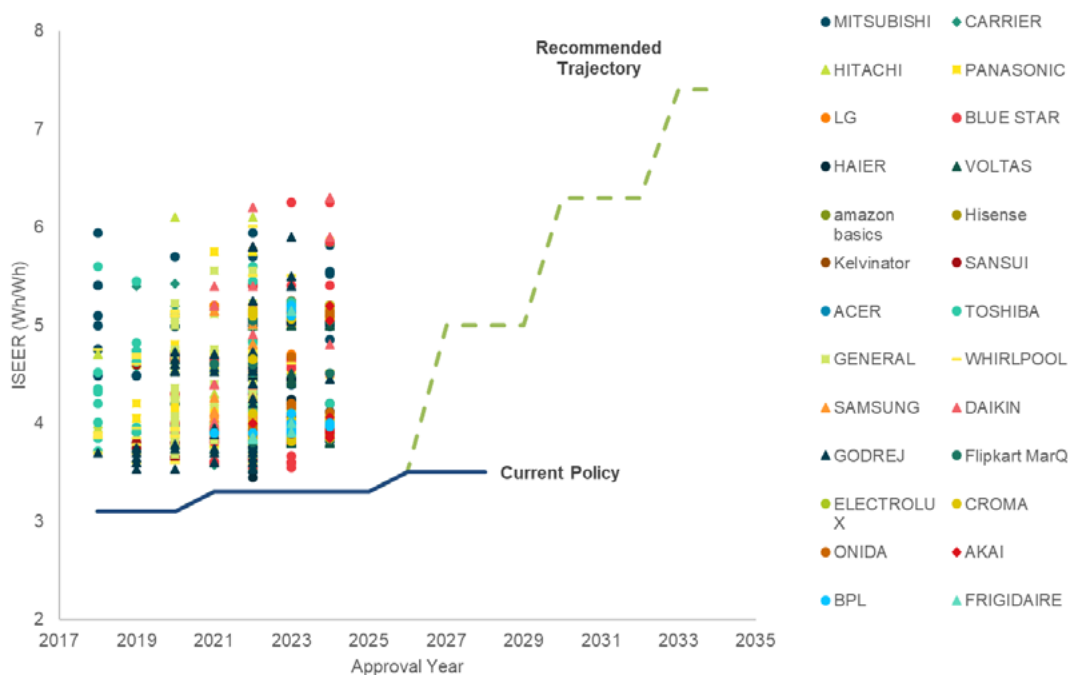
FIGURE 19: Recommended trajectory for room AC (variable speed) 1-star label (green line). The chart also shows BEE's current policy as well as historical 1-star levels (black line).
